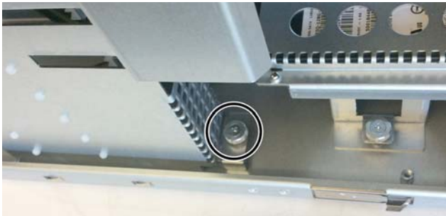
Figure 5. E6L card bracket thumbscrew
