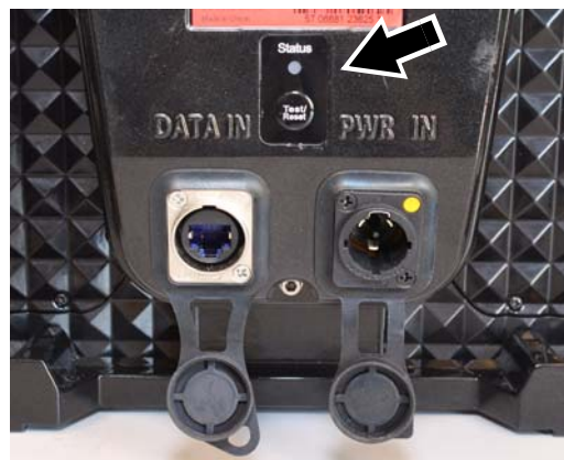
Figure 38: Test/reset button and status indicator LED
