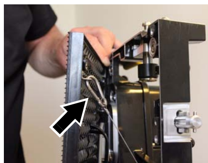
Figure 39: Replacing an LED block, rear access
